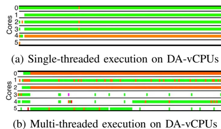
Fig. 2: Linux load balancing is unaware of vCPU asymmetry
